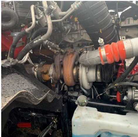
S13 truck, right side of engine, turbo charge
